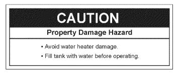
Never use this water heater unless it is completely full of water. To prevent damage to the tank and heating element, the tank must be filled with water. Water must flow from the hot water faucet before turning "ON" power.
